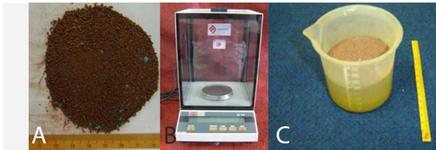
Figure 1: Red granulated phenolic resin (280g) were weighed in a digital analytical balance.
