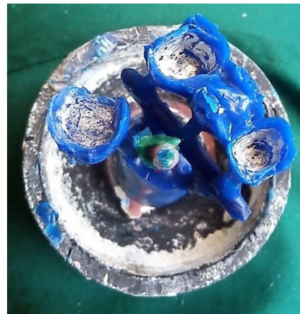
Figure 19 - Laboratory Procedure - Sprue Attached to the Sprue Former.
