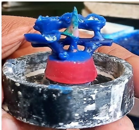
Figure 18 - Laboratory Procedure - Sprue Attachment.
