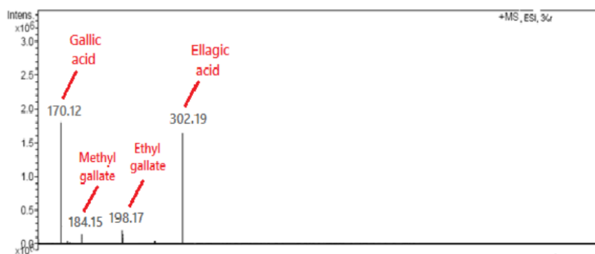
Fig. 4.11: LCMS analysis of fruit extract of Terminalia chebula showing the peaks of Gallic acid, Methyl gallate, Ethyl gallate and Ellagic acid.
